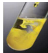
Figure 10.3 Precipitation of \text{PbI}_2
