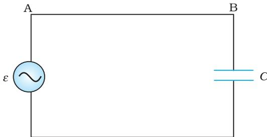
**FIGURE 7.7** An ac source connected to a capacitor.
