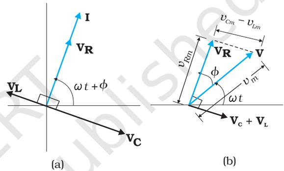
**FIGURE 7.11** (a) Relation between the phasors  $\mathbf{V}_L$ ,  $\mathbf{V}_R$ ,  $\mathbf{V}_C$ , and  $\mathbf{I}$ , (b) Relation between the phasors  $\mathbf{V}_L$ ,  $\mathbf{V}_R$ , and  $(\mathbf{V}_L + \mathbf{V}_C)$  for the circuit in Fig. 7.10.
