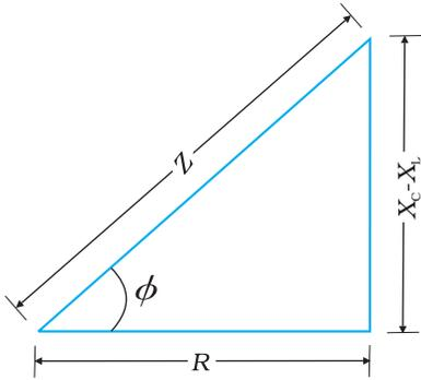
FIGURE 7.12 Impedance diagram.
