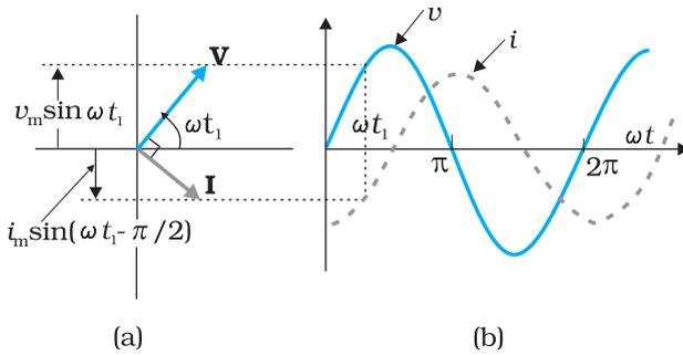
**FIGURE 7.6** (a) A Phasor diagram for the circuit in Fig. 7.5.
