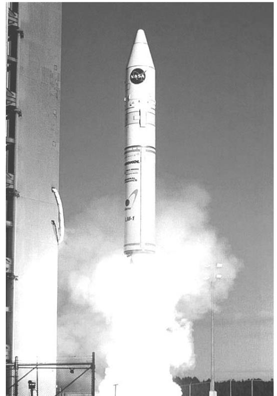
***R**ocket propulsion is based upon the law of conservation of linear momentum. The fuel is burnt in the ignition chamber of the rocket engine. The gases so produced are ejected from an orifice in the rear of the rocket. A thrust acts on the rocket due to reaction of the movement of gases and thus the rocket starts moving in the forward direction.*
