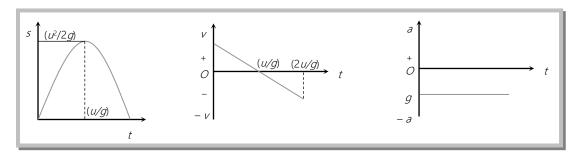
It is clear that both quantities do not depend upon the mass of the body or we can say that in absence of air resistance, all bodies fall on the surface of the earth with the same rate.
