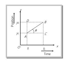
It is clear that slope of position-time graph represents the velocity of the particle.
