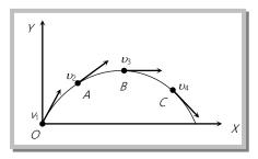
Direction of these velocities can be found out by drawing a tangent on the trajectory at a given point.
