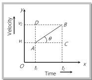
It is clear that slope of velocity-time graph represents the acceleration of the particle.
