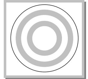
The angular half width of Airy disc =  $\theta = \frac{1.22\lambda}{D}$  (where  $D$  = aperture of lens)
