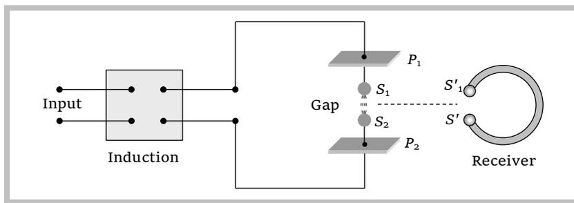
When a high voltage is applied across metallic plates these plates get discharged by sparking across the narrow gap. The spark will give rise to oscillations which in turn send out electromagnetic waves. Frequency of these wave is given by  $\nu = \frac{1}{2\pi\sqrt{LC}}$
