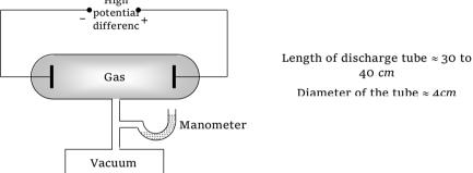
The discharge tube is filled with the gas through which discharge is to be studied. The pressure of the enclosed gas can be reduced with the help of a vacuum pump and it's value is read by manometer.
