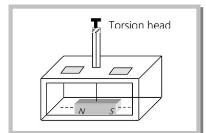
Where,  $I$  = moment of inertia of short bar magnet =  $\frac{wL^2}{12}$  ( $w$  = mass of bar magnet)
