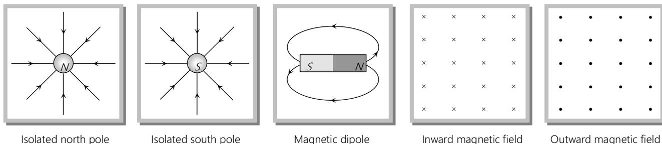
(2) **Magnetic flux ( $\phi$ ) and flux density ( $B$ )**
