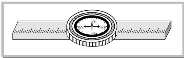
Different position of deflection magnetometer : Deflection magnetometer can be used according to two following positions.
