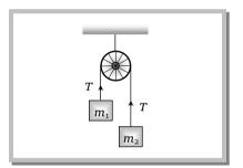
Solution: (b) Tension in the wire  $T = \frac{2m_1m_2}{m_1 + m_2}g$ : stress in the wire  $= \frac{T}{S} = \frac{2m_1m_2g}{S(m_1 + m_2)}$
