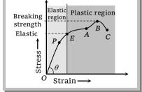
This behaviour is shown up to point E known as elastic limit or yield-point. The region OPE represents the elastic behaviour of the material of wire.
