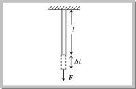
Linear strain in the direction of deforming force is called longitudinal strain and in a direction perpendicular to force is called lateral strain.
