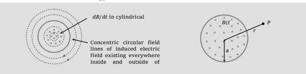
A uniform but time varying magnetic field B(t) exists in a circular region of radius 'a' and is directed into the plane of the paper as shown, the magnitude of the induced electric field ( $E_{\rm in}$ ) at point P lies at a distance r from the centre of the circular region is calculated as follows.
