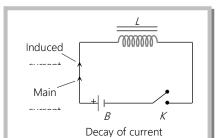
The value of current at any instant of time t after closing the circuit (*i.e.* during the rising of current) is given by  $i = i_0 \left[ 1 - e^{-\frac{R}{L}t} \right]$ ; where  $i_0 = i_{\max} = \frac{E}{R}$  = steady state current.
