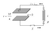
At  $t = \frac{3T}{4}$ , capacitor again discharges completely  $i = i_{max}$
