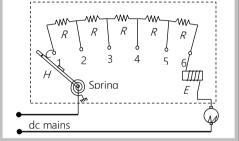
The value of starting resistance is maximum at time t=0 and its value is controlled by spring and electromagnetic system and is made to zero when the motor attains its safe speed.
