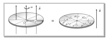
A metal disc can be assumed to made of uncountable radial conductors when metal disc rotates in transverse magnetic field these radial conductors cuts away magnetic field lines and because of this flux cutting all becomes identical cells each of emf 'e' where  $e = \frac{1}{2}B\omega r^2$ , as shown in following fig. and periphery of disc becomes equipotential.
