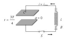
At  $t = \frac{3T}{4}$ , capacitor again discharges completely  $i = i_{max}$
