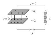
At t = 0, capacitor is ready to discharge
