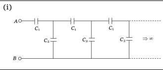
Suppose the effective capacitance between A and B is  $C_R$ . Since the network is infinite, even if we remove one pair of capacitors from the chain, remaining network would still have infinite pair of capacitors, i.e., effective
