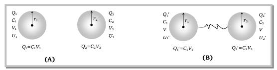
(i) **New charge**: According to the conservation of charge  $Q_1 + Q_2 = Q_1' + Q_2' = Q$  (say), also  $\frac{Q_1'}{Q_2'} = \frac{C_1 V}{C_2 V} = \frac{4\pi\varepsilon_0 r_1}{4\pi\varepsilon_0 r_2}$ ,  $\frac{Q_1'}{Q_2'} = \frac{r_1}{r_2}$   $\Rightarrow$   $1 + \frac{Q_1'}{Q_2'} = 1 + \frac{r_1}{r_2}$   $\Rightarrow$   $\frac{Q_1' + Q_2'}{Q_2'} = \frac{r_1 + r_2}{r_2}$
