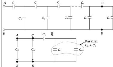
Suppose there are n sections between A and B and the network is terminated by  $C_0$  with equivalent capacitance  $C_R$ . Now if we add one more sections to the network between D and C (as shown in the following figure), the equivalent capacitance of the network  $C_R$  will be independent of number of sections if the capacitance between D and C still remains  $C_0$  i.e.,
