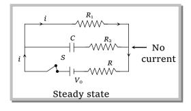
When capacitor gets fully charged (steady state), no current flows through the line in which capacitor is connected. Therefore the current through resistor  $R_1$  is  $\frac{V_0}{(R_1+r)}$ , hence potential
