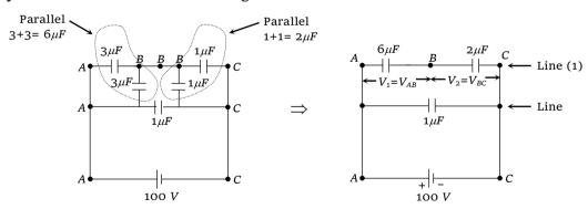
By using the formula to find potential difference in series combination of two capacitor
