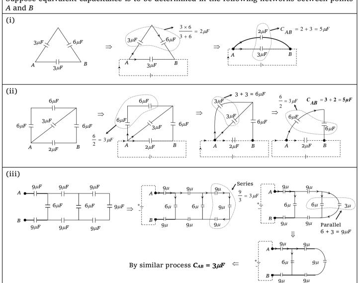
(2) Circuits with extra wire: If there is no capacitor in any branch of a network then every point of this branch will be at same potential. Suppose equivalent capacitance is to be determine in following cases
