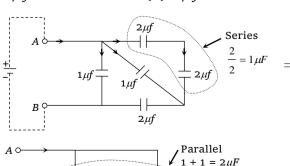
$A \circ \longrightarrow \bigvee_{\substack{1 \mu f \\ 1 \neq 1 \\ 2 \mu f}} Parallel \\ 1 + 1 = 2 \mu F$
