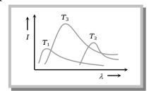
Solution: (b) According to Wien's law  $\lambda_m \propto \frac{1}{T}$  and from the figure  $(\lambda_m)_1 < (\lambda_m)_3 < (\lambda_m)_2$  therefore  $T_1 > T_3 > T_2$ .
