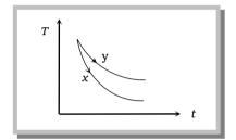
Solution: (c) From the graph it is clear that initially both the bodies are at same temperature but after that at any instant temperature of body x is less then the temperature of body y. It means body x emits more heat *i.e.* emissivity of body x is more than body y :  $e_x > e_y$
