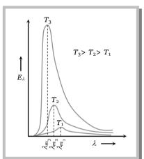
intensity of radiation at a particular temperature. This area increases with rise in temperature of the body. It is found to be directly proportional to the fourth power of absolute temperature of the body, *i.e.*,
