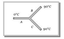
Solution: (b) Let the conductivity of each rod is K. By considering the rods B and C are in parallel, effective thermal conductivity of B and C will be 2K.
