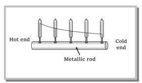
After sometime, a state is reached when the temperature of every cross-section of the rod becomes constant. In this state, no heat is absorbed by the rod. The heat that reaches any cross-section is transmitted to the next except that a small part of heat is lost to surrounding from the sides by convection & radiation. This state of the rod in which no part of rod absorbs heat is called steady state.
