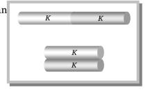
**Problem** 11. Three rods made of the same material and having the same cross section have been joined as shown in the figure. Each rod is of the same length. The left and right ends are kept at  $0^{\circ}C$  and  $90^{\circ}$  respectively. The temperature of the junction of the three rods will be
