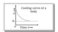
*i.e.*, if the temperature of body is not very different from surrounding, rate of cooling is proportional to temperature difference between the body and its surrounding. This law is called Newton's law of cooling.
