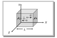
After rebound this molecule travel toward opposite wall  $A_2$  with velocity  $-v_x$ , collide to it and again rebound with velocity  $v_x$  towards wall  $A_1$ .
