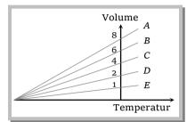
Solution: (d) From  $PV \propto MT$  or  $V \propto \frac{M}{P}T$ ; Here  $\left(\frac{M}{P}\right)$  represents the slope of curve drawn on volume and temperature axis.
