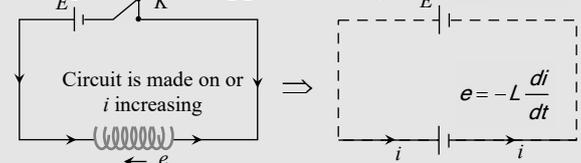
Sometimes at sudden opening of key, because of high inductance of circuit a high momentarily induced emf produced and a sparking occurs at key position. To avoid sparking a capacitor is connected across the key.
