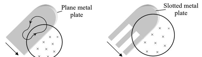
(A) Strong eddies produced Cause excessive electro magnetic damping
