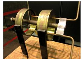
(1) **Principle** : It is based on the fact that a current carrying coil placed in the magnetic field experiences a torque. This torque rotates the coil.
