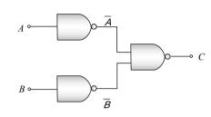
$C = \overline{\overline{A}.\overline{B}} = \overline{\overline{A} + \overline{B}} = A + B \qquad \text{(De morgan's theorem)}$
