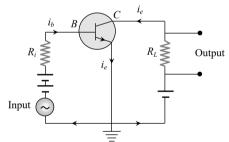
This has been shown a *NPN* transistor. Therefore base emitter are forward, biased and input signal is connected between base and emitter.
