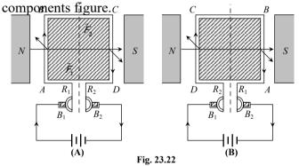
ABCD = Armature coil,  $S_1$ ,  $S_2$  = split ring comutators
