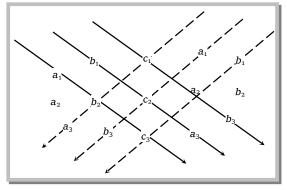
Taking product of R.H.S. diagonal elements positive and L.H.S. diagonal elements negative and adding them. We get the value of determinant as  $= a_1b_2c_3 + b_1c_2a_3 + c_1a_2b_3 - c_1b_2a_3 - a_1c_2b_3 - b_1a_2c_3$
